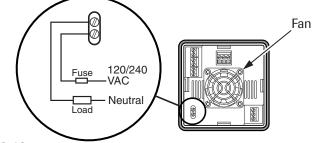
Figure 3.12 Control Output Wiring–T5 and T10
